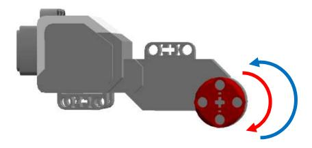
To make the robot turn , adjust the Steering setting: the block will control the speed and direction of both the motors to make the robot turn
